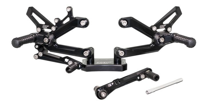
This set is pre-assembled. Remove the factory set and mount the ARP racing parts rear set in place of the original set. We recommend torquing the M8 screws to 20-22 Nm and the M6 screws to 10 Nm. Make sure you tighten all of the parts after adjusting. We highly recommend using a low to medium strength threadlocker (our recommendation is Loctite 222). You are done, let's race!
