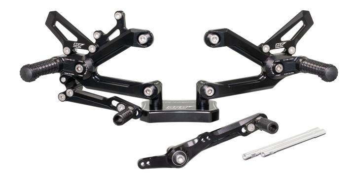
This set is pre-assembled. Remove the factory set and mount the ARP racing parts rear set in place of the original set. We recommend torquing the M8 screws to 20-22 Nm and the M6 screws to 10 Nm. Make sure you tighten all of the parts after adjusting. We highly recommend using a low to medium strength threadlocker (our recommendation is Loctite 222). You are done, let's race!
